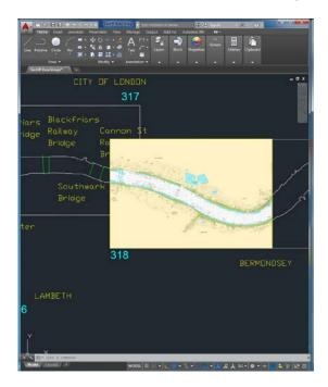
Now you can bring in other CAD drawings rescale and rotate them and create products on PLA charts as well as the drawings being in the correct spatial location. (NOTE: DXF is in meters so drawings should be scaled accordingly)
