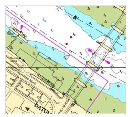
River users should note that temporary stake boat moorings will be established on the start line of the Boat Race course from approximately 0900 and recovered on conclusion of the practice starts. These will be positioned upstream of Putney Bridge centre arch, as marked in red on the chartlet, and marked by pellet buoys. The distance between these pellet buoys will be 18m and mariners are to navigate with caution in their vicinity.
