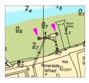
4.2.A.19. **Woolwich Reach**: 2x Fixed Red Navigation Lights on Barrier Gardens Pier to be removed, as the pier currently has three sets lights. Upriver and downriver sets to be retained and the middle set removed.
