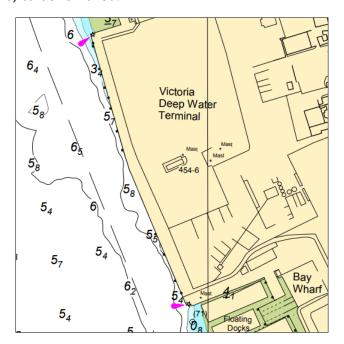
4.2.A.14. **Bugsby's Reach**: 4x Fixed Red Navigation Lights on the Cable Car lights (N19395/60) to be removed, as they are directly below and inshore of North Greenwich Pier.
