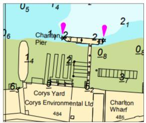
4.2.A.18. **Woolwich Reach**: 4x Fixed Red Navigation Lights on Riverside Wharf to be removed, as they are over a drying area and set back from the Authorised channel.
